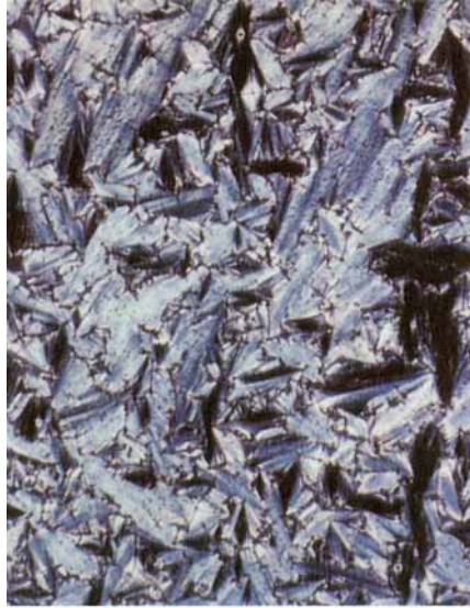
Figure 7. Broken focal conic fan texture of polymer IC at 23°C (after the sample has undergone a crystallization transition).
