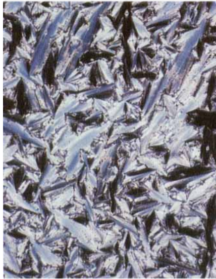
Figure 6. Smectic A focal conic fan texture of polymer IC at 160°C.
