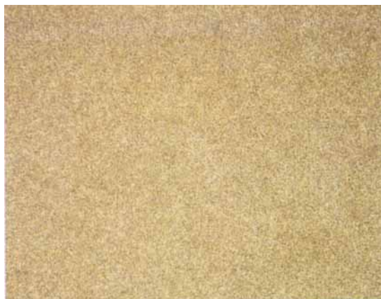
Figure 8. Grainy smectic A texture of a sample of polymer IC after flash cooling the isotropic liquid.
